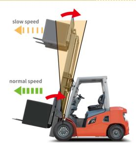
Mast speed control function: When working at a high position, the mast's rear tilt speed is intelligently controlled, and the front and rear tilt ends are intelligently buffered to maintain stability during high-altitude operations.
