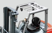
The overall stamping design of the cab offers enhanced safety protection.
